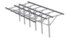
Fig. 3.3.4: Mounting structure
