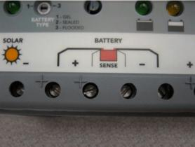
Fig. 2.3.26: Battery voltage sensing of a charge controller
